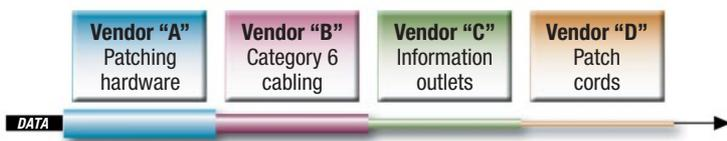
If not perfectly matched, components can reflect data signals where they join. Even if each component is Category 6 compliant, end-to-end performance can be greatly reduced.
